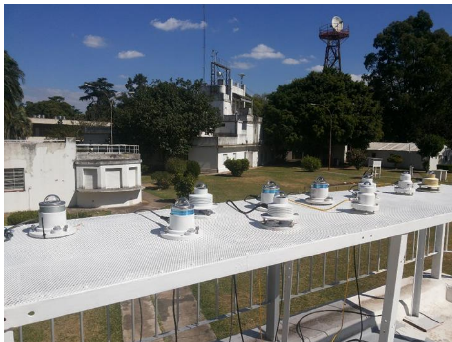
Figure 4. UV radiometers installed in the calibration platform in order to ensure that the irradiance received is the same.
