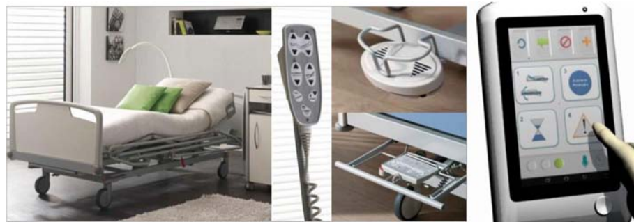
Fig. 4 User interfaces in smart beds are multiple, robust and dedicated to the patient and/or caregiver. Integration of new technologies, ergonomics and graphical interfaces allows for improved control over a broader range of functions. Left: Olympia Hospital bed, developed and manufactured by Haelvoet [46]. Right: example of a graphical-user interface designed for the control of a new generation of medical beds [47]. Permission for use of images granted by Haelvoet
