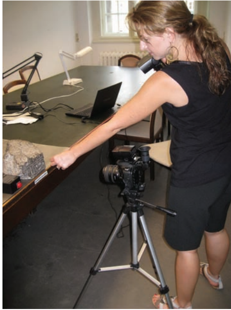
Fig. 3. Moving the flash around an object (Sheshonq I/Abiba'al fragment; KAI 5) at a consistent distance in a typical RTI photo shoot. Vorderasiatisches Museum, Berlin (VA 3361). (Image by Heather Dana Davis Parker and Johanan Daniel Church Davis)
