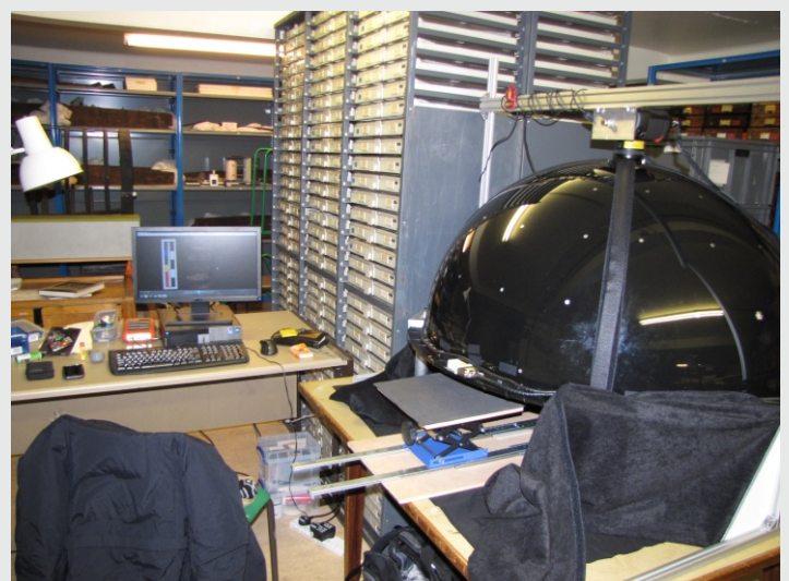
Figure 1. Reflectance Transformation Imaging camera and lighting dome system. Left: Dome being assembled in the Centre for the Study of Ancient Documents at the University of Oxford. The front dome quarter is removed to show the array of 76 LED light sources. Right: The RTI dome system set up ready for imaging in the British Museum Blythe House Stores. Lights and camera (suspended from metal frame over dome) are connected to the PC which controls these and the RTI capture process. Author's photographs.
