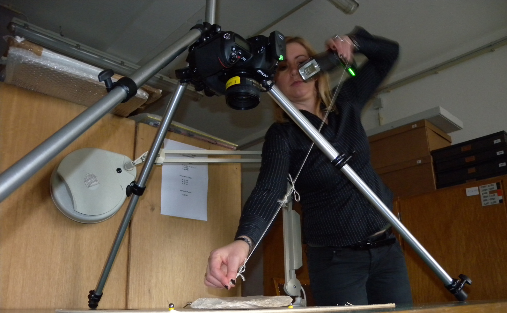
Figure 2. H-RTI equipment set up for the capture of a limestone ostrakon in the Ägyptisches Museum und Papyrussammlung, Staatliche Museen zu Berlin. The author measures the distance between the flash gun and target surface prior to taking one of a series of digital photographs. Photograph courtesy Hembo Pagi.
