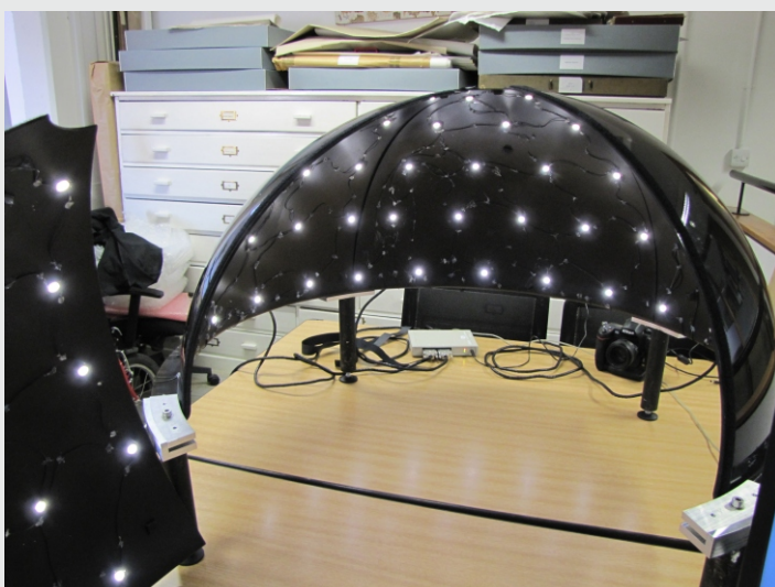
Figure 1. Reflectance Transformation Imaging camera and lighting dome system. Left: Dome being assembled in the Centre for the Study of Ancient Documents at the University of Oxford. The front dome quarter is removed to show the array of 76 LED light sources. Right: The RTI dome system set up ready for imaging in the British Museum Blythe House Stores. Lights and camera (suspended from metal frame over dome) are connected to the PC which controls these and the RTI capture process. Author's photographs.
