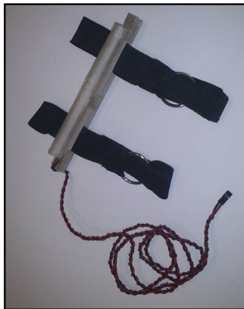
Figure 1. Linear cylindrical optical marker with two elastic clamps and power cable.
