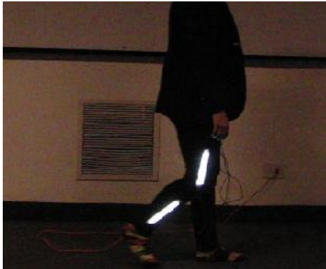
Figure 3. Video frame of a subject under study, with markers in lower limb, from which the pre-processing stage begins.
