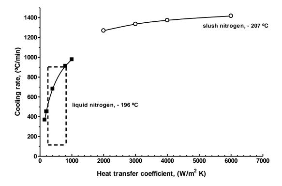
Figure 2. Comparison of calculated cooling rates for French straw corresponding to liquid nitrogen conditions (-196°C, h  $\leq$  800) with conditions assumed for slush nitrogen (-207°C, h  $\geq$  2000). The rectangle indicates probable range of h values for film boiling regime.
