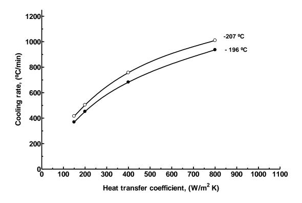
**Figure 1.** Comparison of calculated cooling rates for French straw at -196°C and -207°C in a range of heat transfer coefficients estimated to be representative of film boiling.
