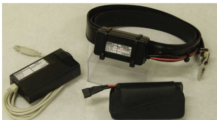
Figure 1. System components: Wearable sensing terminal (top), battery pack (bottom right), and USB base (left).
