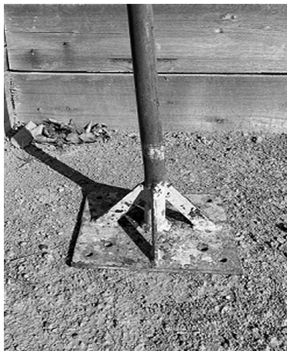
Figure 3. Image of the compaction tool with 4 kg mass dropped three times from a height of 0.30 m onto an area of 0.20 m × 0.17 m.
