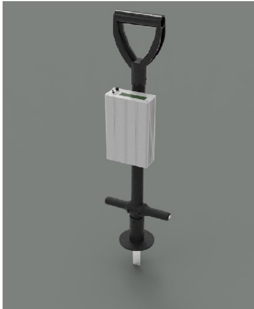
Figure 4. A drawing of the two axis commercial strain-gauge sensor, the Going Stick.
