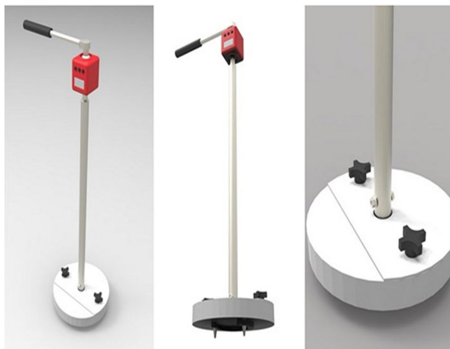
Figure 6. The rotational traction tester based on a device used for playing fields (ASTM F2333-04).
