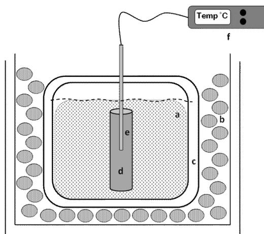
**Figure 1.** a) The dry ice-ethanol liquid bath, b) air/styrofoam pellet insulation, c) styrofoam insulation, d) PTFE or PMMA cylinder, e) type T copper-nickel probe fit snug into the drilled cylinder, f) data acquisition system. Dry ice-ethanol bath was prepared by addition of dry ice chips during stirring until system reached a stable temperature of  $-78^{\circ}\text{C}$ .
