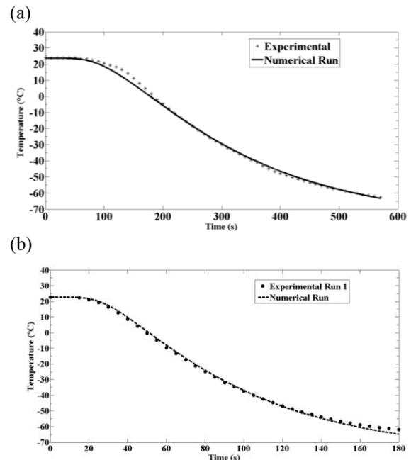
**Figure 2.** Predicted and measured center temperature of PMMA cylinder 1.30 cm diameter (a) and of PTFE cylinder 2.59 cm diameter (b) immersed
