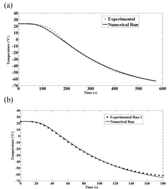
**Figure 2.** Predicted and measured center temperature of PMMA cylinder 1.30 cm diameter (a) and of PTFE cylinder 2.59 cm diameter (b) immersed in a dry ice-ethanol cooling bath.
