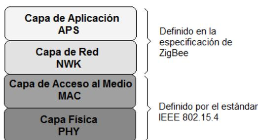
Figura 2.1: Pila de protocolos ZigBee/802.15.4
