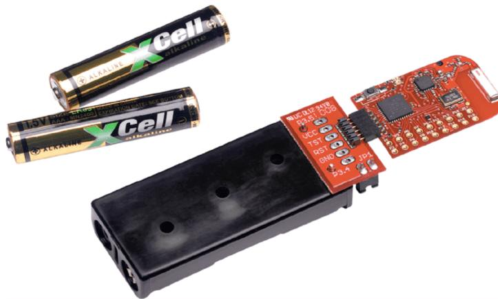
Figura 3.14: ez430-RF2500: target board.
